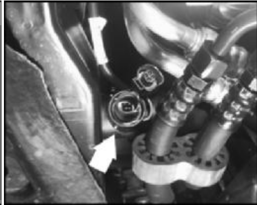
F54 Coolant fan control (FC) thermal switch
