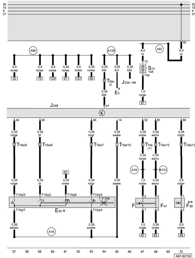
**Diesel direct injection system control unit, cruise control system switch, brake light switch**
